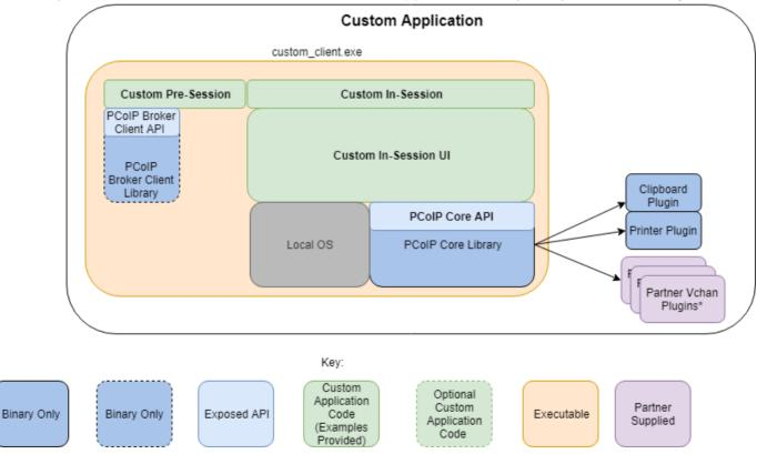
This diagram shows the architecture with a custom application integrating the core library.
